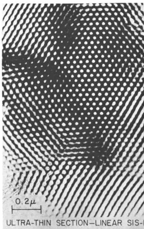
Figure 9. TEM of a styrene-isoprene styrene triblock copolymer
